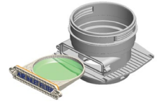
Air Intake Filter (installed)
